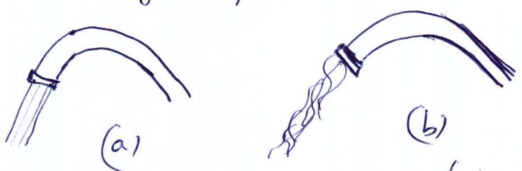
Turbulences are induced by irregularities (defects) roughness of the pipe, etc... They are damped out at low speeds but conserved and amplified at larger speeds.
