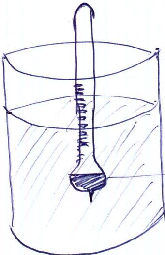
$\rightarrow$  the weight at the bottom makes the scale float upright.
