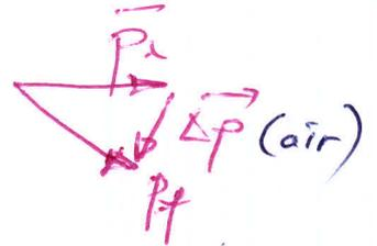
equivalent explanation: wing imparts a net downward momentum to the air, so reaction force is upward.
