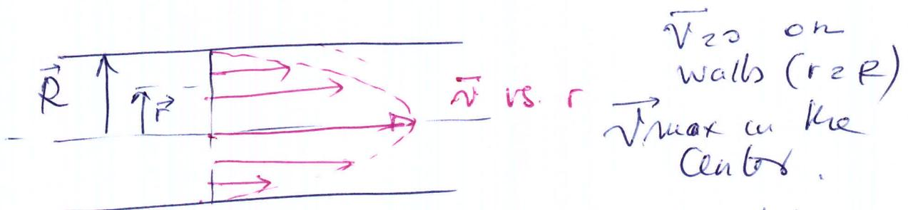
The motion is like a lot of concentric tubes sliding relative one another, with the central tube moving fastest and the outer tube at rest.
