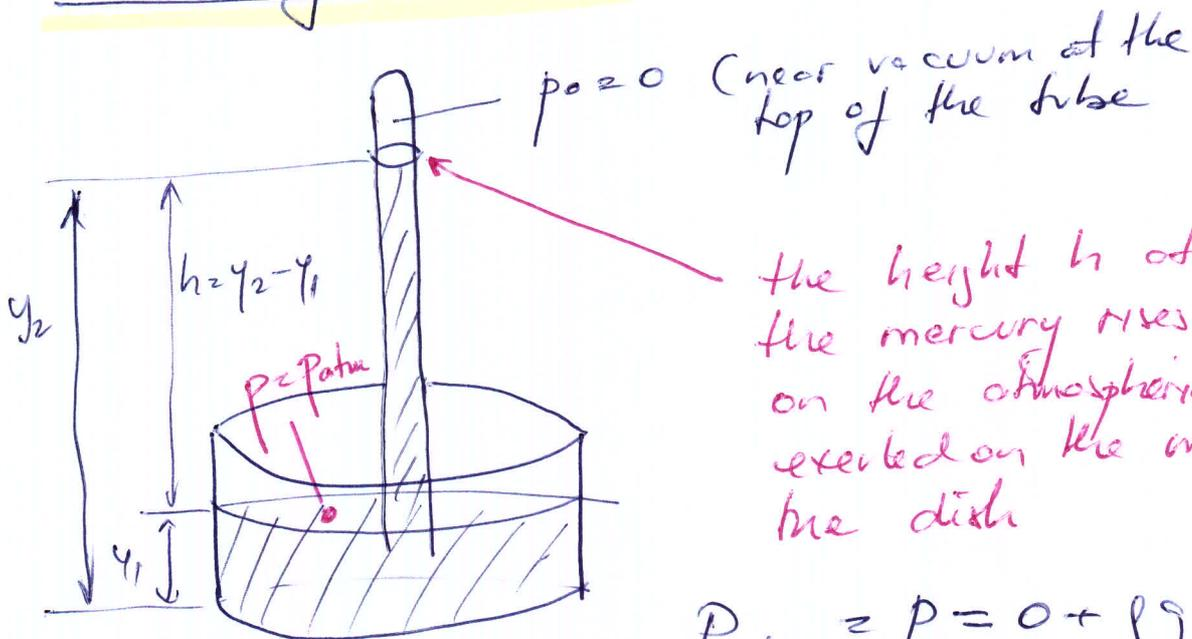
the height  $h$  at which the mercury rises depends on the atmospheric pressure exerted on the mercury in the dish
