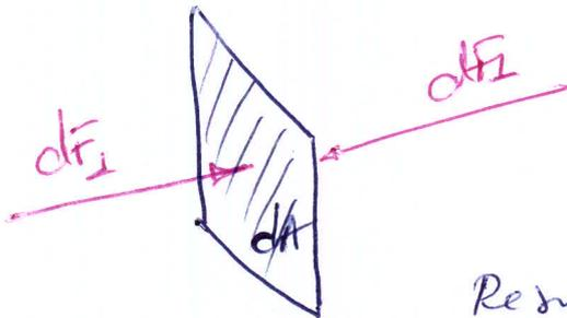
a small surface  $dA$  within a fluid at rest.
