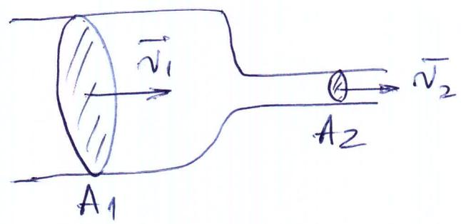
$$dm_1 = dm_2 \quad ; \quad \rho A_1 v_1 dt = \rho A_2 v_2 dt$$
