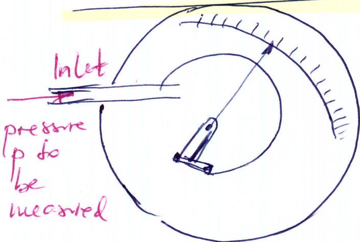
Changes in the inlet pressure cause the tube to coil or uncoil which moves the pointer
