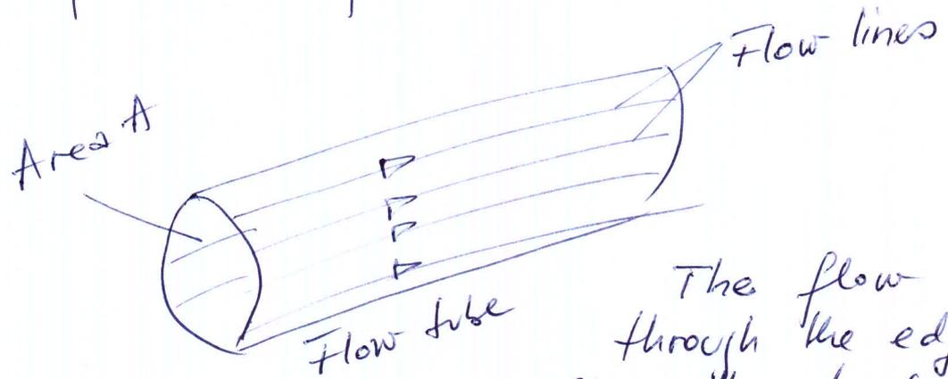
The flow lines passing through the edge of an imaginary element of area A form a flow-tube.
