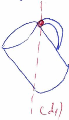
suspend the ring at point A; the line (d1) passes CG.
