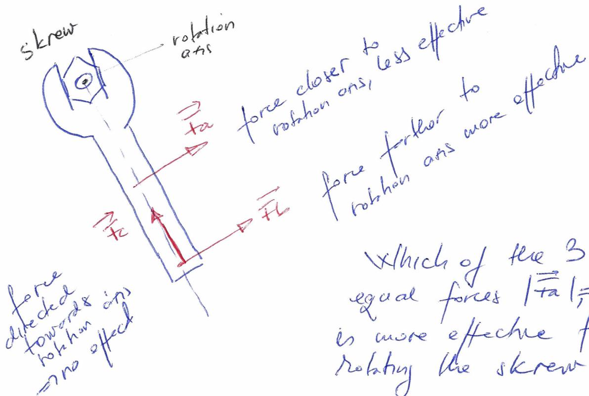
Which of the 3 equal forces  $|\vec{F}_a|, |\vec{F}_b|, |\vec{F}_c|$  is more effective for rotating the skewer?
