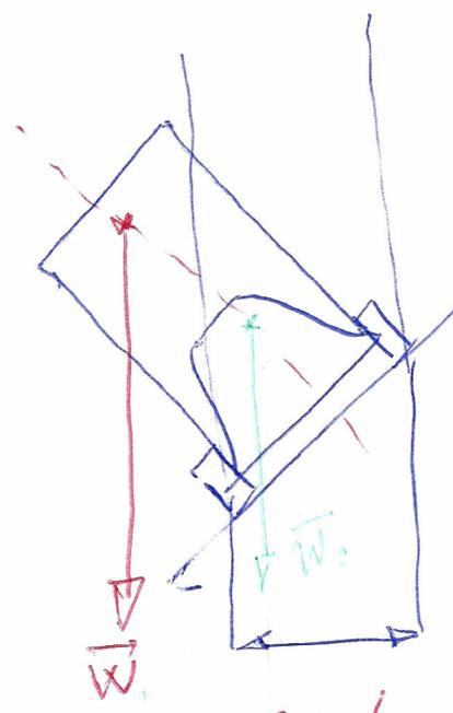
the higher the CG, the smaller the incline needed to overturn the vehicle
