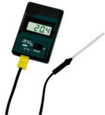
Thermocouple (Seebeck effect)
