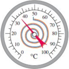
(c) A bimetallic strip used in a thermometer
