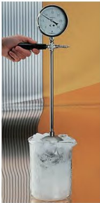
(a) A constant-volume gas thermometer
