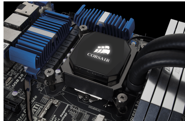
Water cooling of processor
