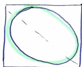
In case when the amplitude ratio changes, the slope changes for the rectangle inscribing the ellipse
