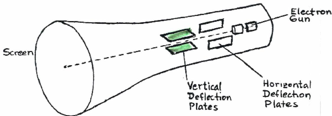
Working principle: deflection of an electron in electric field  $\vec{F} = q\vec{E}$
