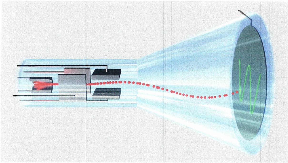
We will apply on x input:  $X = U_x \sin(\omega_x t)$  and on Y input:  $Y = U_y \sin(\omega_y t + \varphi)$  using two signal generators with variable frequencies and amplitudes.
