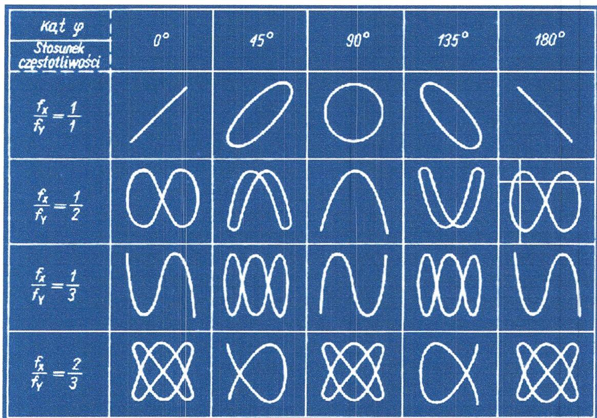
Engineers can use the principles of Lissajous figures to precisely tune and set up the phase relation between a known reference signal and a signal to be tested.
