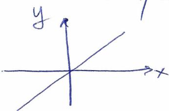
The interference of two perpendicular oscillations with same frequency and in-phase ( $\varphi=0$ ) leads to an harmonic oscillation along a linear direction
