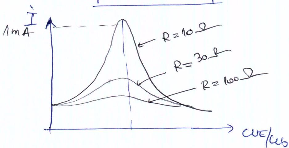
$$\begin{aligned} L &= 100 \mu H \\ C &= 100 \mu F \\ E &= 10 mV \end{aligned}$$
