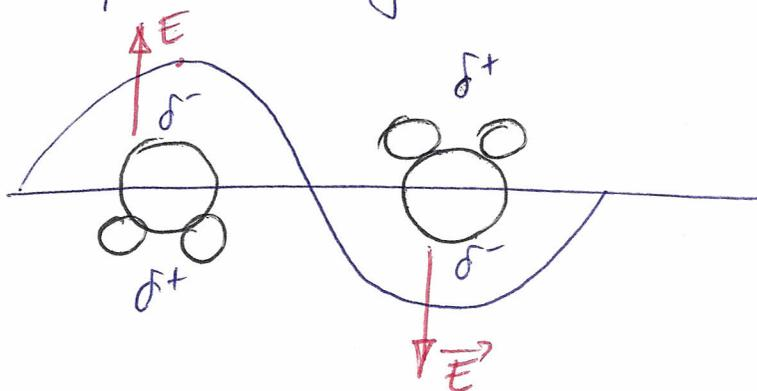
dipole positions where the electric force due to  $\vec{E}$  is zero.
