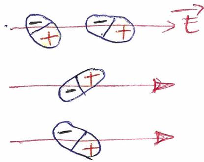
Then, the polar molecules tend to be aligned with the external electric field
