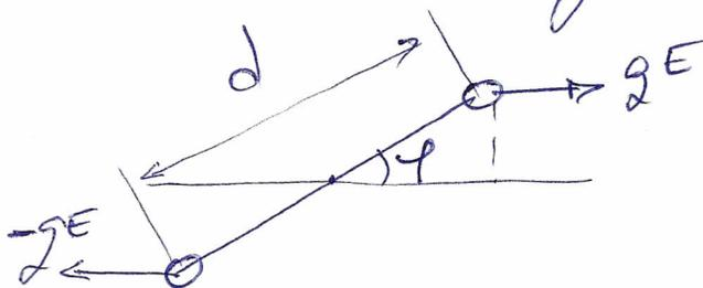
$$\boxed{p = qd} \Rightarrow \text{electric dipole moment} \quad \underline{[p] = C \cdot m}$$
