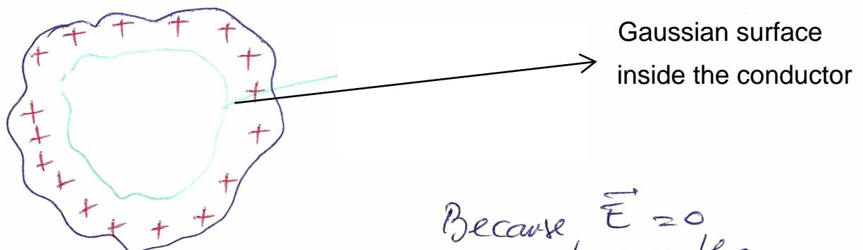
cross-section of conductor
