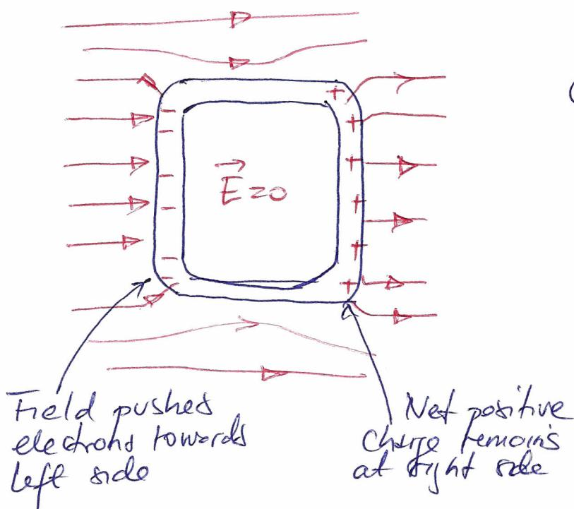
Conducting box immersed in external electric field
