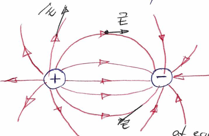
at each point  $\vec{E}$  is tangent to the field line passing through the electric point
