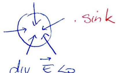
describes the net flow going in vs. going out for a vector field. In absence of creation or destruction of matter the identity within a region can change only by having it flow into or out of the region.  $\rightarrow$  principle of continuity fundamental in Physics
