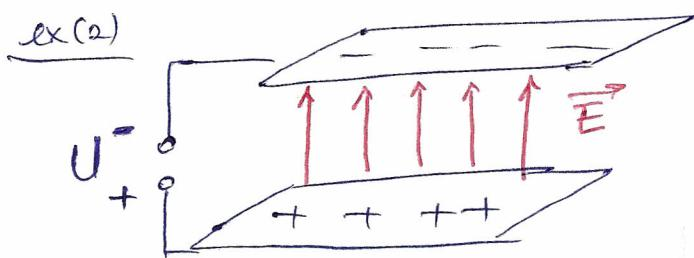
uniform electric field between two parallel conducting plates connected at a battery
