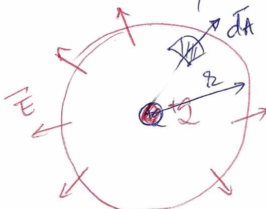
Gaussian spherical surface around a positive charge
