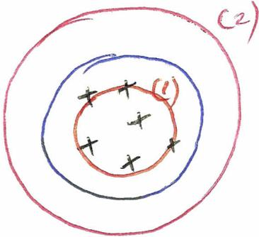
To calculate the electric field we consider a Gaussian surface spherical of radius  $r$  in the two situations  $r < R$  and  $r > R$ .
