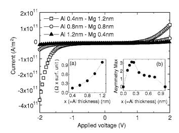
FIG. 2. Computed current density as a function of applied voltage in a composite  $Al_2O_3(x \text{ nm})/MgO(1.6 \text{ } x \text{ nm})$  tunnel junctions for x=1.2 nm, 0.8 nm, and x=0.4 nm. Inset (a), variation of the area resistance as a function of x; inset (b), variation of the maximum current asymmetry as a function of x.
