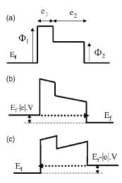
FIG. 1. Composite tunnel barrier potential profile at zero applied voltage (a), under a positive applied voltage (b), and under a negative applied voltage (c).
