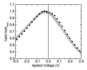
FIG. 8. Measure of the normalized TMR as a function of applied voltage at 300 K in a composite Al(0.7 nm)/Mg(1.6 nm) tunnel barrier with  $t_{\rm Ox}$  equal to 48 s (- $\bigcirc$ -) and in a composite Al(0.7 nm)/Mg(1.1 nm) tunnel barrier with  $t_{\rm Ox}$  equal to 20 s (- $\bigcirc$ -).
