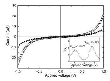
FIG. 7. Current as a function of applied voltage in a composite Al(0.7 nm)/Mg(1.6 nm) tunnel barrier with  $t_{\rm Ox}$  equal to 48 s measured at 300 K (-O-) and 77 K (- $\bullet$ -). Inset: calculus of the  $\hat{I}(V)$  also on the same junction.
