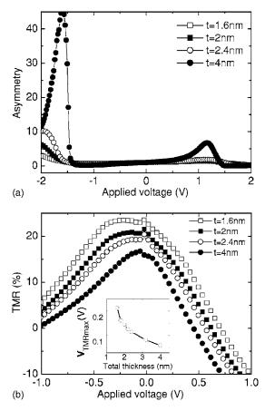
FIG. 4. (a) Calculated variation of current asymmetry with applied voltage for  $Al_2O_3[(3t/4) \text{ nm}]/MgO[(t/4) \text{ nm}]$  tunnel junctions for t=1.6 nm, 2 nm, 2.4 nm, and 4 nm. (b) Calculated variation of magnetoresistance with applied voltage for  $Al_2O_3[(3t/4) \text{ nm}]/MgO[(t/4) \text{ nm}]$  tunnel junctions for t=1.6 nm, 2 nm, 2.4 nm, and t=4 nm. Inset: variation of  $V_{\text{TMR max}}$  as a function of t.
