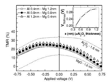
FIG. 3. Computed variation of the tunnel magnetoresistance, TMR, as a function of applied voltage in a composite  $Al_2O_3(x \text{ nm})/MgO(1.6 \text{ } x \text{ nm})$  tunnel junctions for x=1.2 nm, 0.8 nm, and x=0.4 nm. Inset: variation of  $V_{\text{TMR max}}$  as a function of x. The TMR(V) for single 1.6 nm thick  $Al_2O_3$  and MgO barriers have been added in as dotted lines in the figure.
